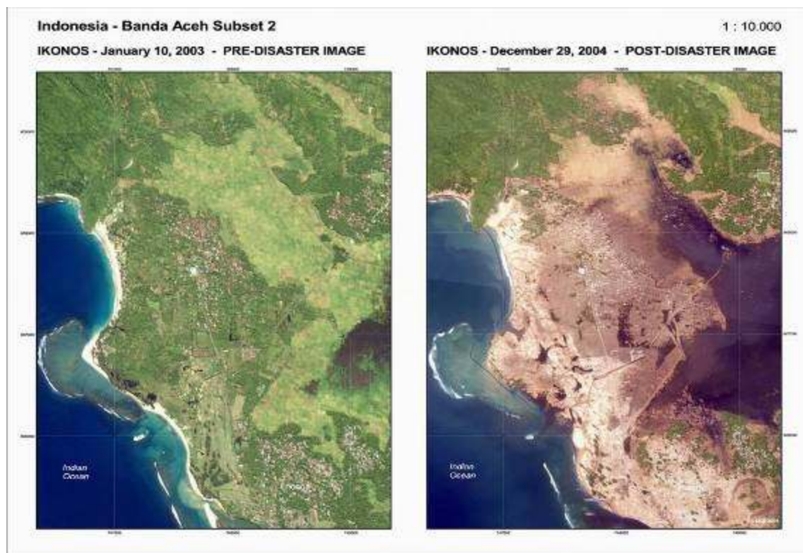
Figure 16. Ikonos imagery of tsunami damage in Banda Aceh showing pre-tsunami (January 2003) and post-tsunami (December 2004) views. Post-tsunami image clearly shows extent of water inundation on land and resulting terrestrial damage (Image printed with the permission of the Respond Consortium).
